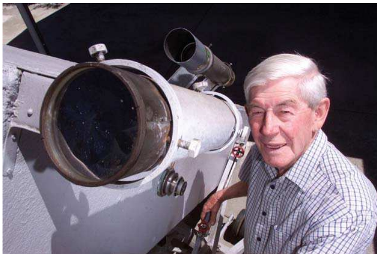
Figure 10. The 78mm & 45mm finder telescopes on 'Lesbet'. Jones used these not only as finder 'scopes but also for observing the variable stars that were too bright for the primary telescope.
