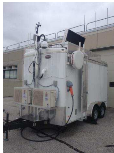
Figure 9: Arctic aerosol/water vapour Lidar to be installed fall 2016.
