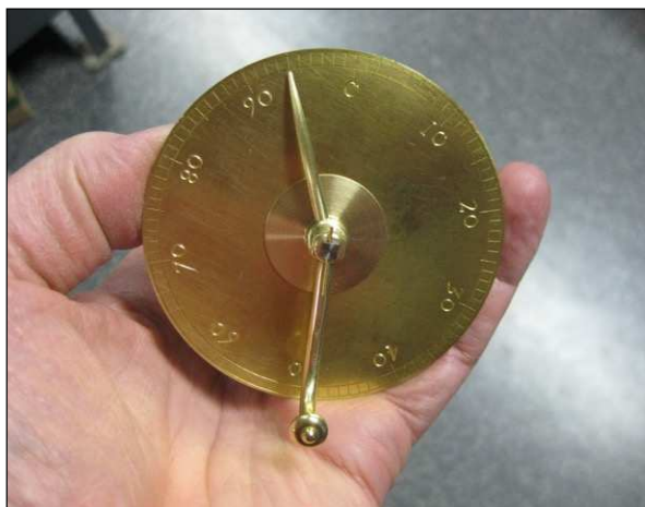
Fig. 3a and 3b: Dial plate, spring plate, and dial pointer hub fixing detail. Compression of the spring plate provides friction which prevents unwanted rotation of the screw and also gives additional end-shake protection.
