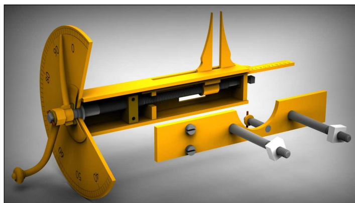
Fig. 2: Cutaway computer visualization of the replica micrometer.
