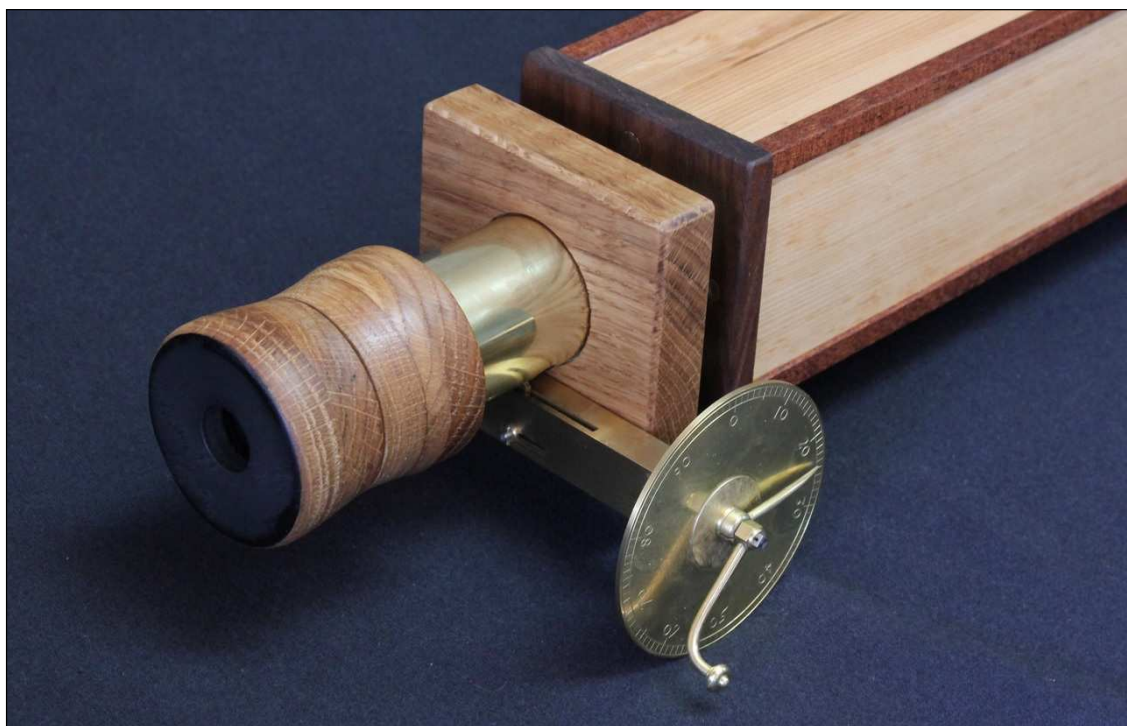
Fig. 5: The telescope mounting method. The two steel threaded pegs riveted to the micrometer brass cover fit into oversize slots in the square oak block, which provides the ability to adjust the position of the micrometer in the light path.
