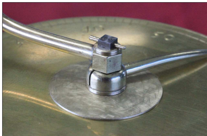
Fig. 3a and 3b: Dial plate, spring plate, and dial pointer hub fixing detail. Compression of the spring plate provides friction which prevents unwanted rotation of the screw and also gives additional end-shake protection.
