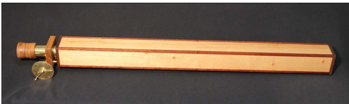
Fig. 7: The tube assembly. The 970 mm case of the telescope is approximately the same length as that used by Gascoigne.
