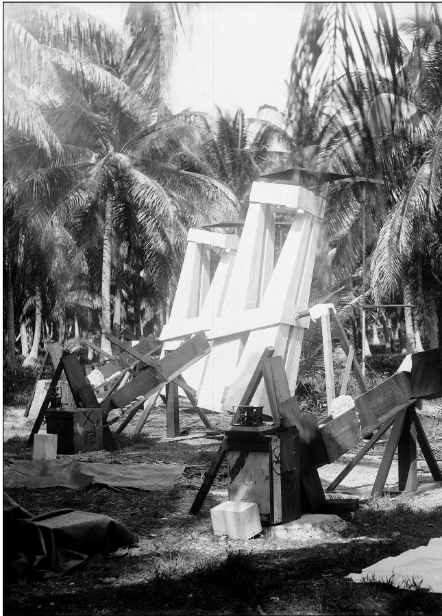
Fig. 7: Lick Observatory eclipse instruments set up on Flint Island, South Pacific, in 1908. Two of the four-barreled cameras first used for the 1905 expeditions can be seen in the background. Lick's director W. W. Campbell felt that the negative result from Flint put the Vulcan question to rest. (Lick Observatory)
