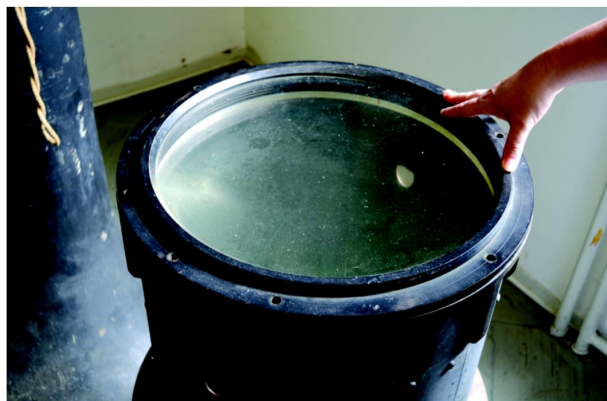
Figure 1 — One of the two original 40-cm aperture f/5 Petzval objective lenses of the Bruce double astrograph. The design consists of four lenses in groups of two. These lenses operated between 1900 and 1950, and allowed the discovery of nearly 500 asteroids (photo by author).
