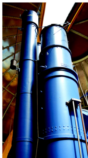
Figure 2 — The Bruce double astrograph in its original dome at the Landessternwarte Königstuhl. The guide telescope is to the left, with one astrograph clearly visible on the right, and the second slightly visible in the gap (photo by author).
