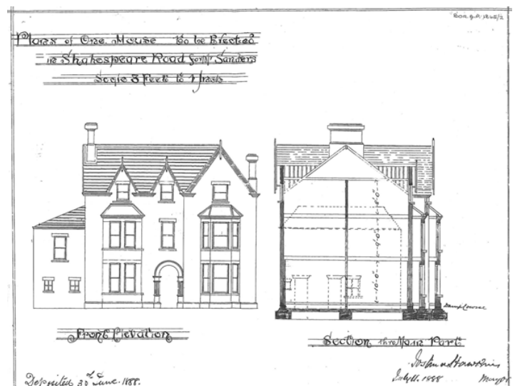
Figure 8. Elevational drawings and cross section of a property to be built on Shakespeare Road for a Mr Saunders. The drawing is dated 1888 and perhaps reflects the general style of houses being built at the time (courtesy the Bedford & Luton Archives and Records Services).
