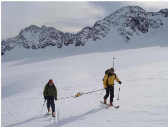
Figure 7. GPR measurement of winter snow depth and internal snow layers on Mittelbergferner, 9 January 2013.
