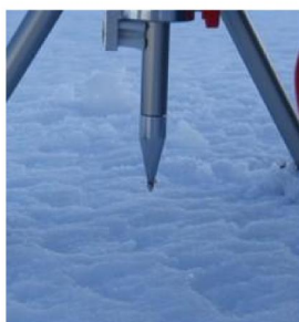
Figure 10. Cone of the SnowMicroPen.
