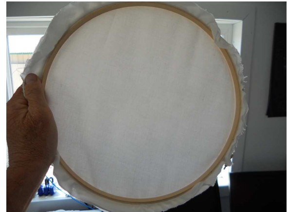
Image 4. One of the two light diffusers used in the early APASS flat system.
