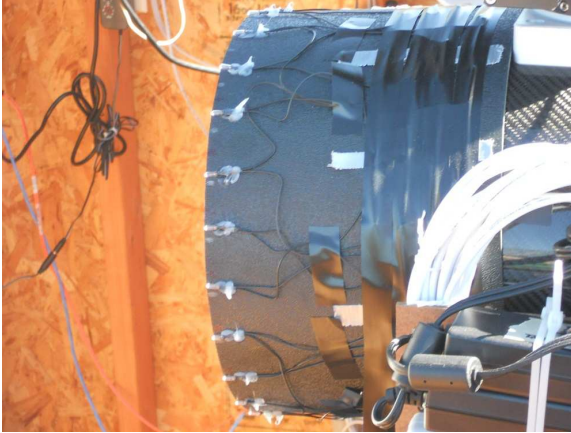
Image 2. One of the OTA flat-field target illumination bank systems with tungsten “grain of wheat” bulbs.
