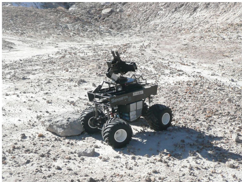
Fig. 4. Rover used for navigation tests, reconnaissance and EVA assistance (courtesy Carnegie Mellon University/NASA Ames).
