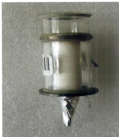
Figure 2. VUV hydrogen glow-discharge lamp
