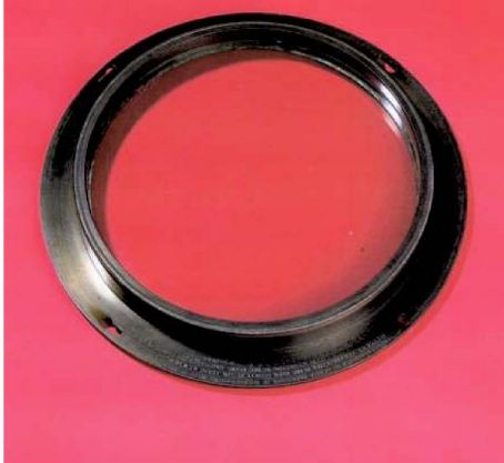
Fig. 6. Huygens' 170-foot focal length object glass. Royal Society MO/1/1/3 and No 23 of 1/010. The object glass appears to have a diameter of about 10 inches.
