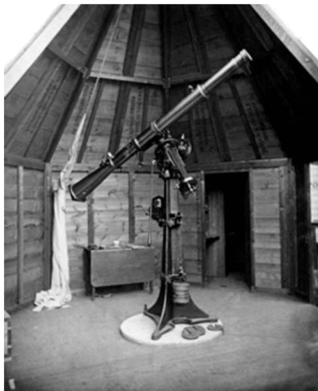
Fig. 21. The photoheliograph used for the 1874 transit of Venus. Royal Astronomical Society ADD MS 93/105.
