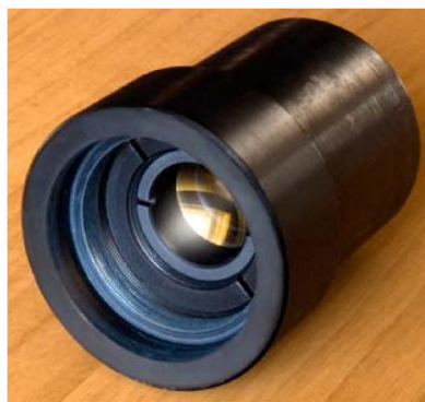
Figure 1. The finished UV corrector.
