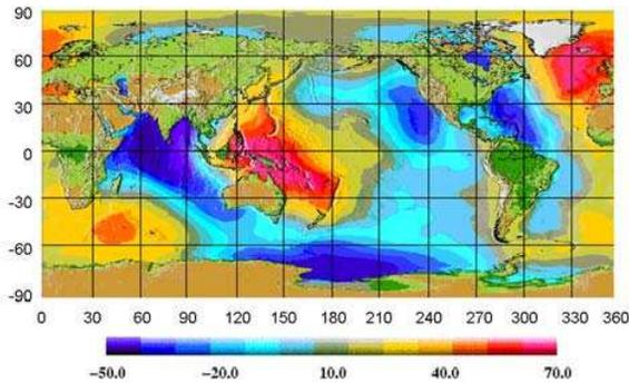
Figure 2. The height (in meters) of the DTU10MSS relative to the WGS84 ellipsoid.
