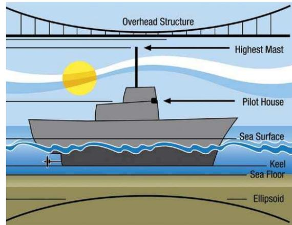
*Figure 1. GPS observations used to navigate the ship gives the 3 coordinates of i.e. the Pilot House or where ever the GPS antenna is mounted. Using this information along with knowledge about the ship, the two clearances are easily determined when the sea surface height and the height of the overhead structure is given relative to the same reference frame. Figure adapted from Maul and Kumar (2005)*
