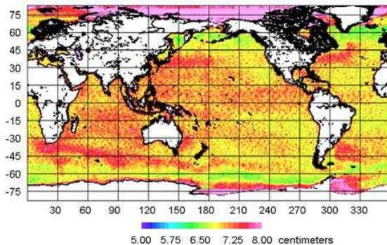
Figure 3. Global interpolation error fields for the DNSC08MSS. The color scale is given in centimeters.
