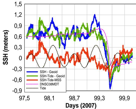
**Figure 7** The GPS observed sea surface height onboard Galathea-3 as the ship sails from 28° N towards Boston crossing the Gulf Stream between day 99.1 and 99.6. GPS heights relative to the geoid without correction for ocean tides are shown in Blue and with ocean tide correction shown in Green. GPS heights relative to the MSS do not contain the Gulf Stream height effect and is shown in Red. The ocean tide effect is shown in Black.
