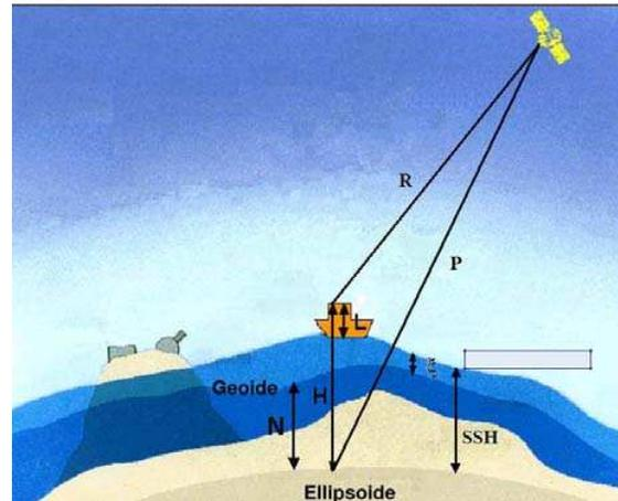
Figure 5 Sea surface height from GPS on-board a ship compared with sea surface height from satellite. GPS measures the height  $H = N+L+\zeta$  relative to the ellipsoid.
