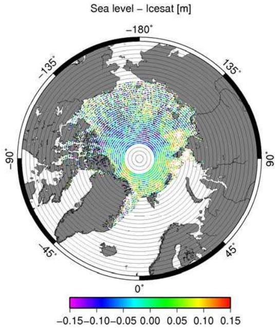
Figure 4.1) The mean difference between 14 months of ICESat laser observations and DTU10MSS. The color scale ranges +/- 15 cm
