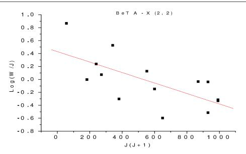
Fig. 7. Plot of log(W/J) vs J(J+1) for BeT A - X (2, 2) band.
