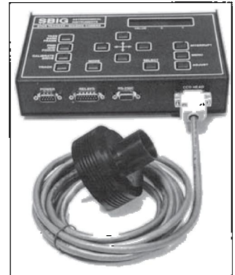
Figure 21. Santa Barbara Instruments Group model ST-4 thermo electrically-cooled CCD camera head and controller.
