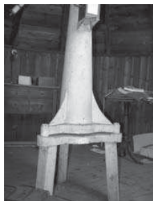
Figure 14. Left: The unusual tripod supporting the telescope pillar. Centre: Close up of the equatorial head. Right: The clock drive mounted just below the equatorial head on the north face of the pillar.
