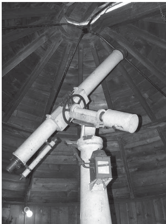
Figure 9. The Troughton & Simms 4-inch f/13 refractor viewed from the north as seen from the trap door into the observatory.
