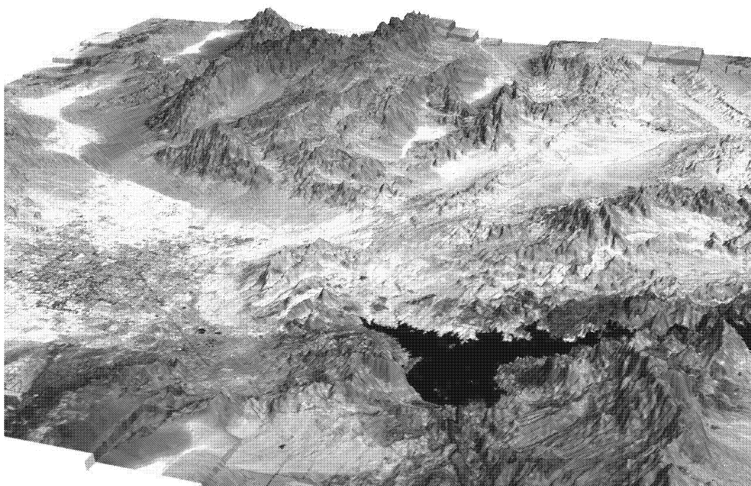
Figure 6: Perspective view of the Las Vegas area created with GRASS (nviz program) based on interferometrically derived heights and a LandSAT image.
