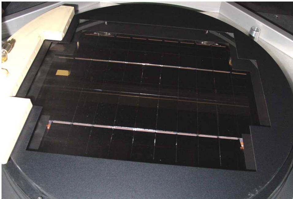
Figure 1. The mosaic of CCD's seen through the entrance windows of the cryostat of MEGACAM, while on its test bench at CEA.
