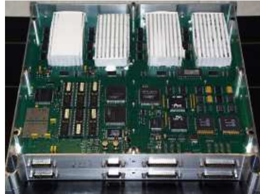
Figure 3: Intel 80386EX-Based OBC and RAMDISK (Top Module Only)
