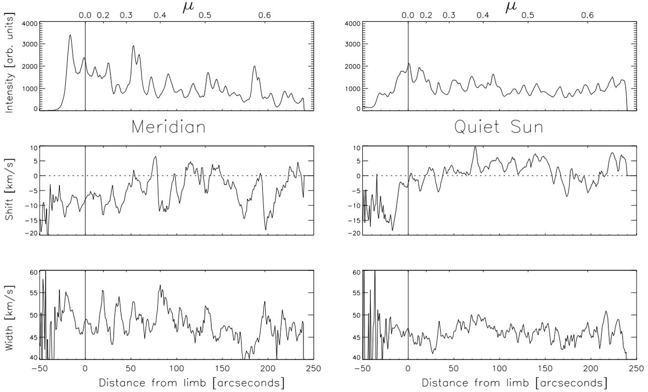
**Fig. 4.** Line parameters (intensity, shift and width) of the spectral profiles of N IV at 765.15 Å obtained in the third set of observations (roll data), averaged over all available data (nine images) in the quiet Sun (right frame) and averaged over all central meridian data (left frame, three images).
