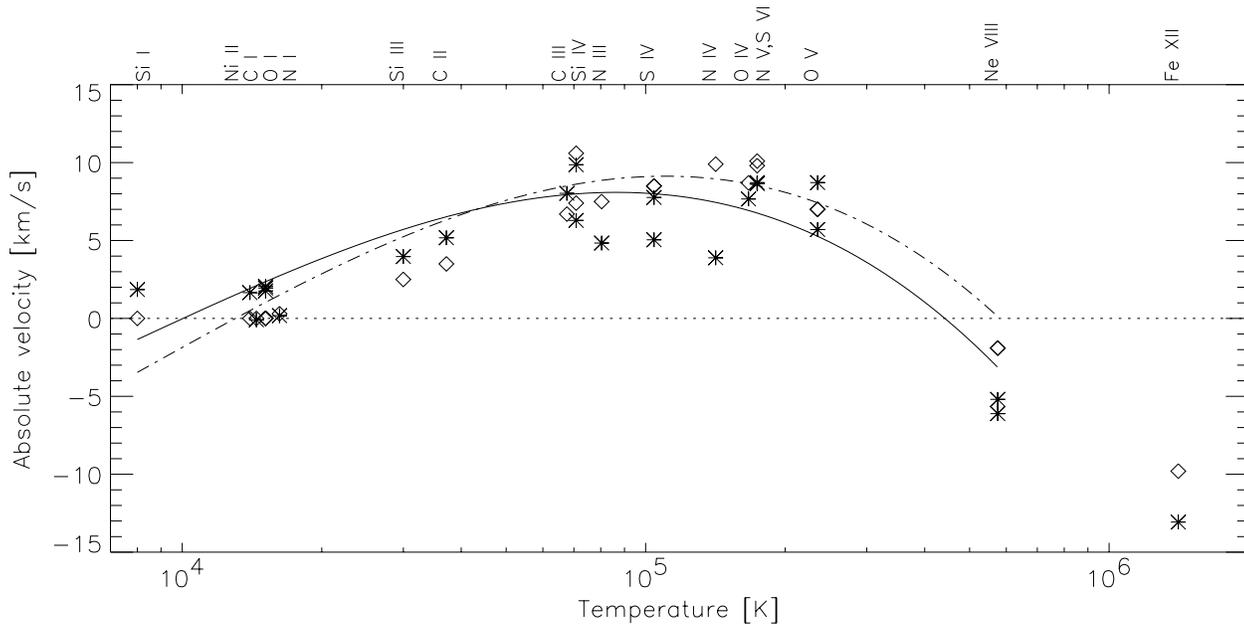
**Fig. 9.** Absolute wavelength shift in velocity units vs. formation temperature. The absolute shifts are determined using the data of Teriaca et al. (1999). Diamonds: large  $\mu$  sector; Stars: small  $\mu$  sector. The solid curve shows a third order polynomial fit to the small  $\mu$  sector points while the dot-dashed curve shows a similar fit to the large  $\mu$  sector points. Negative shifts signify blueshifts.
