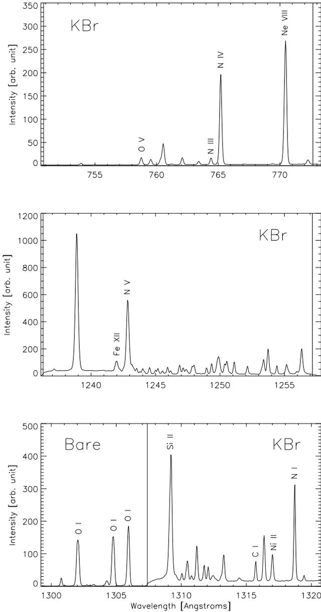
**Fig. 2.** Examples of analysed SUMER spectra. The upper two frames were recorded mainly on the potassium bromide (KBr) photocathode (within the two vertical lines) while the lowest frame shows a spectrum partially recorded on the bare microchannel plate and partially on KBr (separated by the vertical line). The spectra are averaged over the slit length. The analysed lines are identified.
