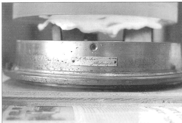
Figure 6: The lens cell was tarnished, pitted and in need of cleaning. The small plaque was difficult to read before being polished; it showed the signature of Brashear, the lens maker. Photo by Brenda Culbertson
