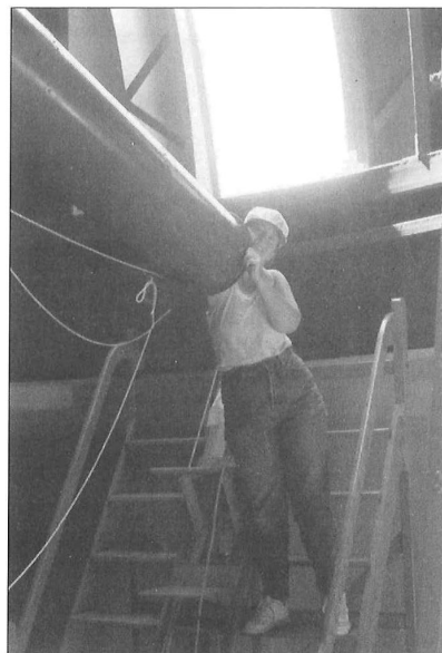
Figure 5: Paint chips were removed from the interior of the tube by Brenda Culbertson during the latest refurbishing project. Mrs. Culbertson spearheaded the refurbishing project fund-raising. Photo by Dr. Ken Ohm.
