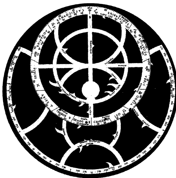
Figure 5. A typical astrolabe rete, courtesy of Harold N. Saunders, All the Astrolabes , Senecio Publishing Company, Oxford, 1984. This is the probable precursor of the planisphere star map. The rete shows the positions of only thirty-three stars. The addition of more stars would make the rete too complicated, and you must remember that it was being used as a clock and not as a guide to the stars. A typical planisphere map would show over 700 stars.
