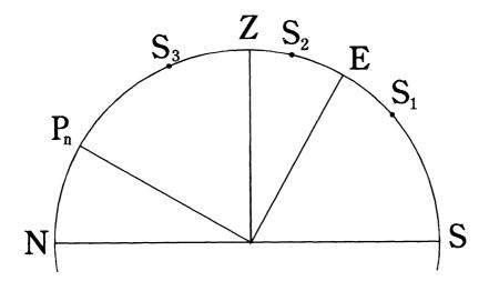
Fig.1. Three possible cases of observation of the Sun's altitude S  $_i$  (i = 1,2,3) at the meridian for latitude determination at sea ( N= North, S=South, Z=Zenith, P = North Pole, E=Equator ).
