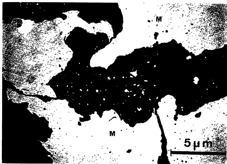
Fig. 8. Backscattered electron image of metal and troilite grains in the host. Sulfide-rich droplets a few to sub- \mu\text{m} in diameter are observed near the larger grains. M: metal, T: troilite.
