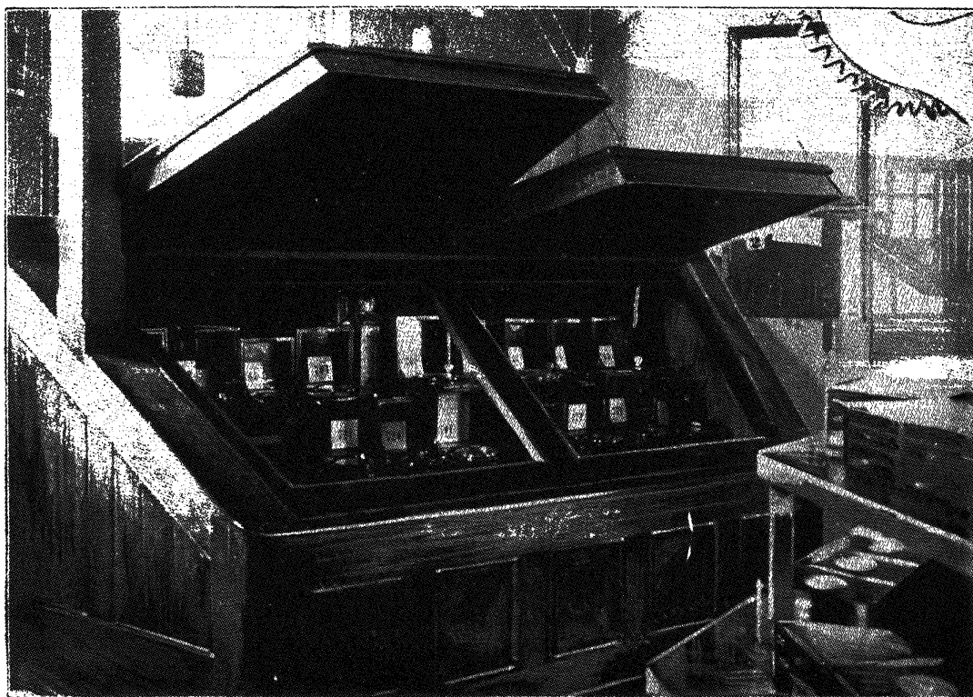
FIG. 2. Throughout Airy's tenure at Greenwich, a considerable fraction of the Observatory's work was devoted to testing of chronometers. The illustration shows the chronometer oven, a device introduced during Airy's time for testing chronometers at varying temperatures. (From Maunder, The Royal Observatory Greenwich , 171.)
