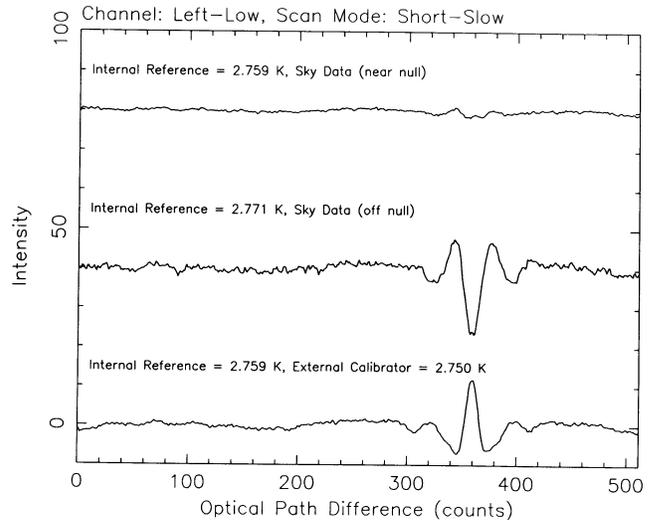
FIG. 1.—Raw co-added interferograms obtained from the FIRAS instrument in flight. *Top*: Sky near null condition, internal reference at 2.759 K; *middle*: sky slightly off-null, internal reference at 2.771 K; *bottom*: external calibrator at 2.750 K, internal reference at 2.759 K. See text for a discussion of thermometer accuracy.
