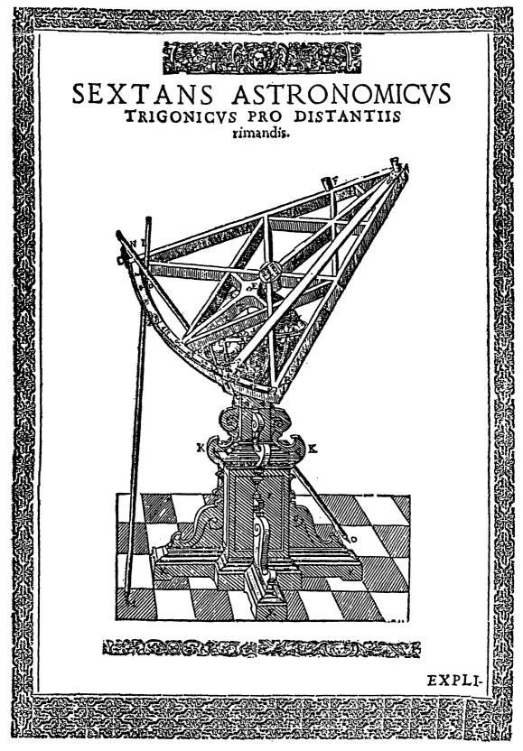
FIGURE 8: Six-foot sextant by ...Mechanica of T.Brahe; note the stabilizing spikes and the ball mounts.
