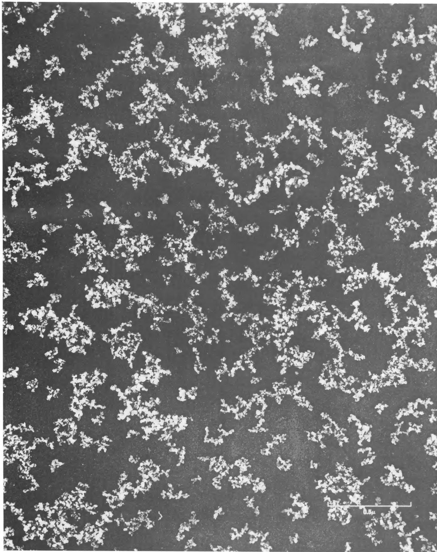
FIG. 1.—Fumed silica clusters. Primary particles are \sim 10 nm. Because of high formation temperature, particles are molten and fuse on contact (courtesy of Cab-O-Sil Division, Cabot Corporation).
