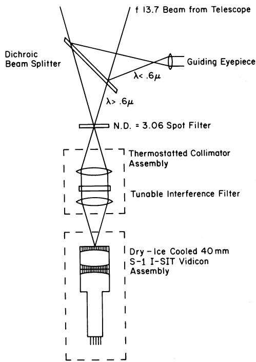
FIG. 1.—The instrumental setup
