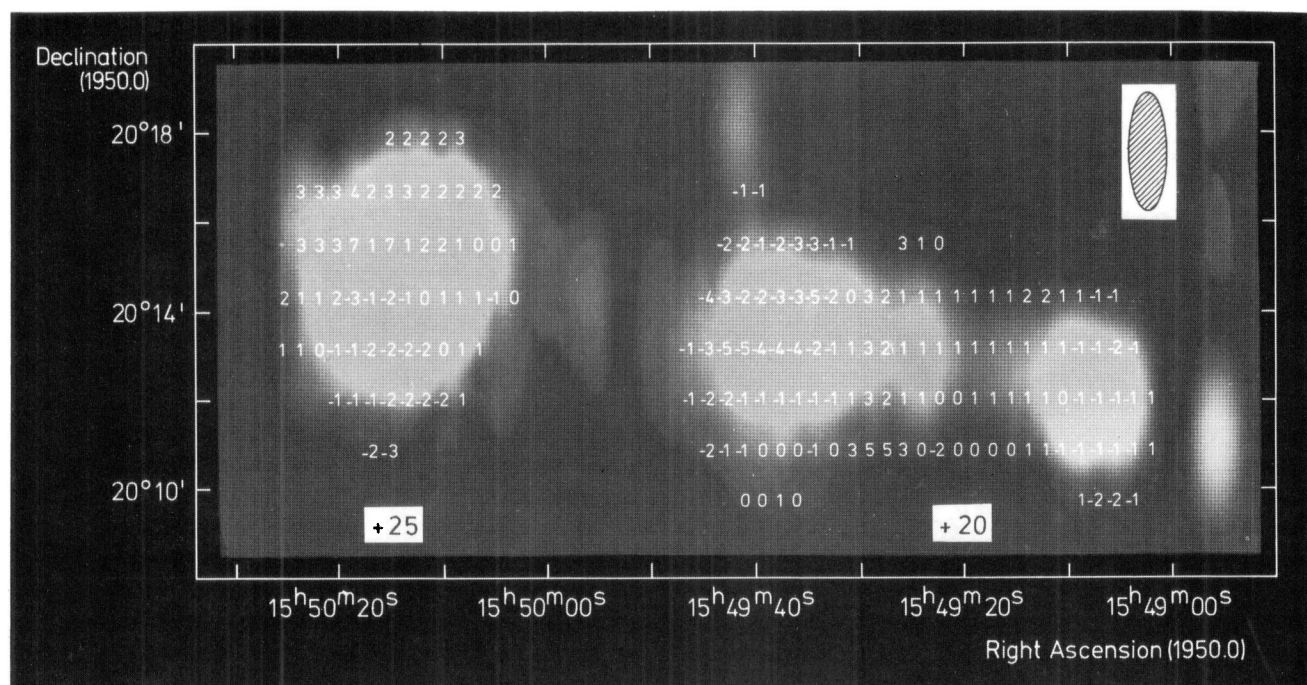
Fig. 8. The distribution of rotation measure over 3C 326 as computed from the 49 cm and 21 cm convolved data superposed upon a “radio photograph” of the 49 cm total intensity. Note that to produce a simple grid of single digit numbers we have subtracted integrated rotation measures, whose derivation is described in the text, of +25 \text{ rad m}^{-2} and +20 \text{ rad m}^{-2} from the values measured at individual sample points in the east and west components respectively. For reference, these integrated values are displayed under each component
