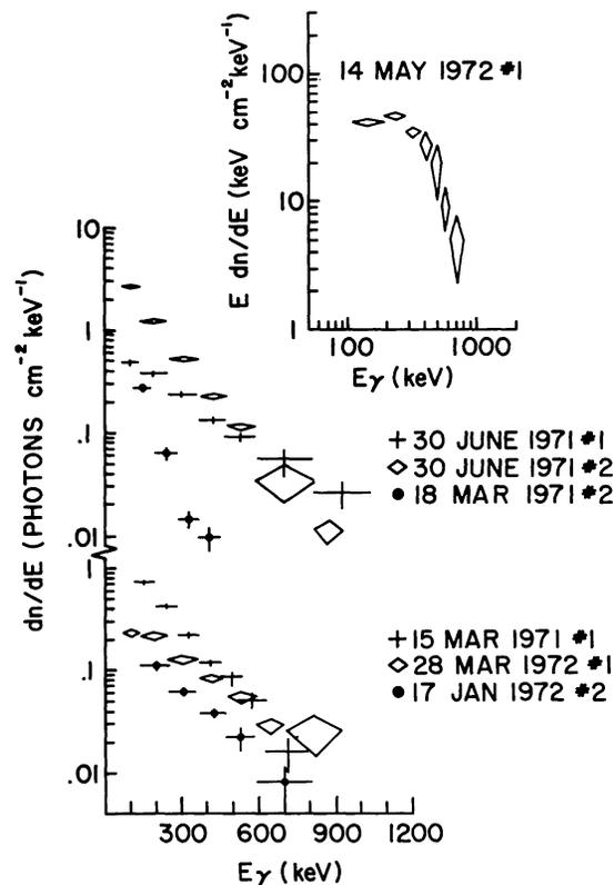
FIG. 2.—(a) Number spectra  $dn/dE$ , of several bursts, selected for the greatest variety of responses. The harder spectra are interpreted as due to attenuation of the incident beam by the satellite material in cases where the source was below the detector horizon (b) (*insert*) The energy spectrum,  $E dn/dE$ , of a directly observed event.
