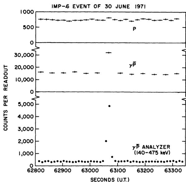
FIG. 1.—The response of the detector to a gamma-ray burst, as indicated by the plastic anti-coincidence (P), the CsI gamma-ray detector ( $\gamma\bar{P}$ ), and several channels added to give the 140–475 keV photon rate, where the gamma-ray energy response is maximized. Each point samples two differential energy spectra.
