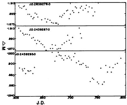
The accompanying figure shows the light curves obtained for three nights. It appears that 20 C Vn is variable with an amplitude of about 0.03 magnitude. The observations are too limited to derive an accurate period or even to establish that the variation is periodic. However, from the individual curves a period of about 0.13 day may be inferred. The light variation and spectral type indicate that 20 C Vn is a Delta Scuti variable.
