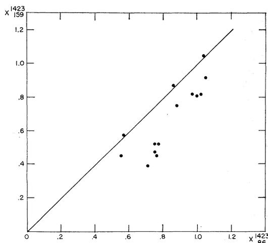
FIG. 3. Comparison of spectral indices determined from two different frequency baselines, for sources where Moffet's observations at 950 Mc indicate no error due to angular size at 159 Mc.
