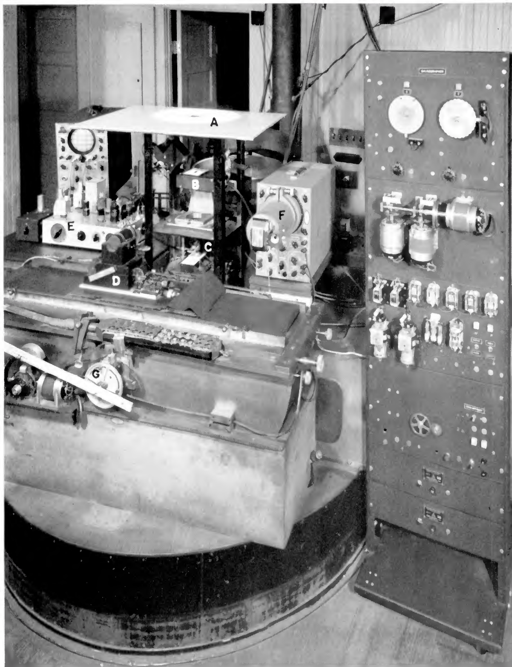
FIG. 8.—The head of the spectrograph, showing (A) image screen, (B) electro-optic retardation plate, (C) Nicol prism above slit, (D) detector, (E) amplifier, (F) recording oscilloscope with camera, and (G) Doppler compensator. At right is rack holding scanning controls and switching circuits. The grating and collimator are at the bottom of the 75-foot pit.
