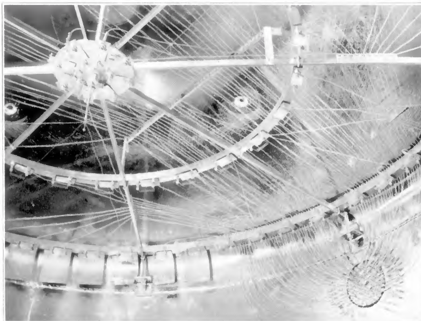
INSIDE VIEW OF THE 108-INCH TANK, SHOWING ELECTRICAL LEADS AT LOWER RIGHT, OUTER ARRAY OF 48 COILS, INTERMEDIATE ARRAY OF 24 COILS, AND CENTRAL ARRAY OF 8 COILS AND ELECTRODE WITH ATTACHED AERIAL FOR ELECTRICAL CLEANING DISCHARGE
