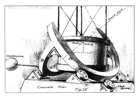
Therefore the yoke is resorted to. The telescope tube is hung between the two bearings instead of outside of them as in Figure *III*, but it will be seen that in order to gain this rigidity a part of the northern heavens has had to be sacrificed. The writer submits a mounting wherein extreme rigidity is found and the entire heavens retained.
