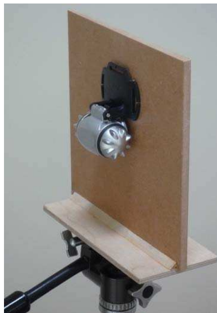
Figure 4. An LED headtorch, bought from a local high street store for £1, makes a convenient light source. Modify it down to one LED, counterbore the MDF board to get the LED as close behind the pinhole as possible and fix it in place with double sided sticky pads.
