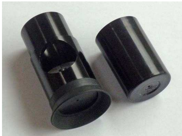
Figure 5. Showing a Cheshire eyepiece alongside a 35mm film canister with a small hole drilled through the exact centre of the base, for use as a collimation eyepiece.
