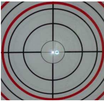
Figure 6. The defocused returned doughnut ring alongside the point source....
