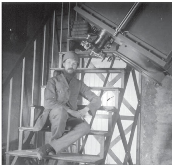
Figure 1. Fernand Baldet at the Pic du Midi telescope in 1909. The eyepiece of the 23cm refractor and the cell of the 50cm mirror are seen at the bottom of the telescope.
