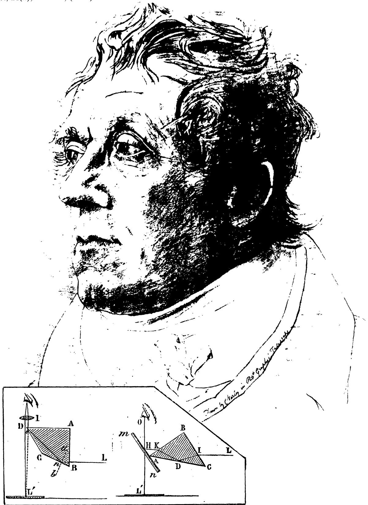
Fig. 330. (a) A sketch by Cornelius VARLEY of the eminent English painter, J.M.W. Turner, made using a graphic telescope which threw an outline on the artist's paper. (b) The camera lucida of WOLLASTON (left) and AMICI (right). W.H.WOLLASTON patented this device c. 1805. It consists of a small prism which is used to effectively divide the pupil - one half then views the object (scenery or a specimen), the other half the drawing being made. AMICI designed a variation in which the head of the drawing pencil was seen projected against the field of view using an additional semi-transparent glass slip.
