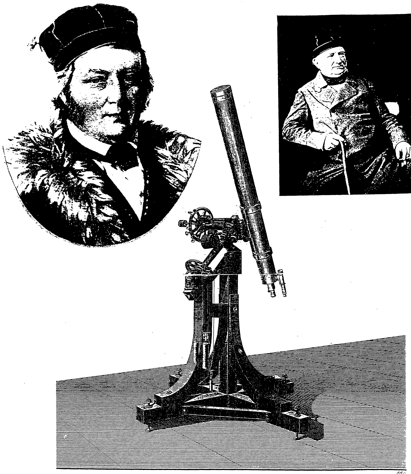
Fig. 308. A small achromatic refractor from the Optical Institute of UTZSCHNEIDER and FRAUNHOFER in Munich, similar to the great Dorpat 9.6-inch FRAUNHOFER refractor (see Cyclopaedia Part 1 , IAJ 20 (3), 181 (1993)) used by STRUVE to measure double stars. Two portraits of the eminent astronomer, F.G.W. STRUVE (1793-1864).
