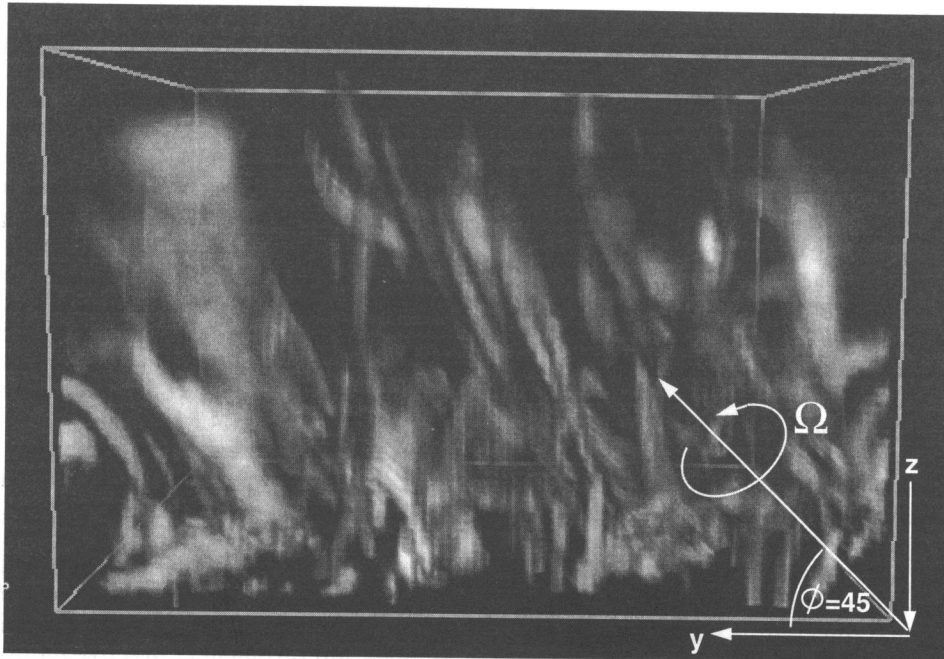
FIG. 11.—Volume rendering of enstrophy as viewed at one instant in time from the side of the layer in simulation R4. In such a strongly rotationally influenced case (with R_0 = 0.71 ), coherent vortex structures align with the rotation vector \Omega over much of the layer.
