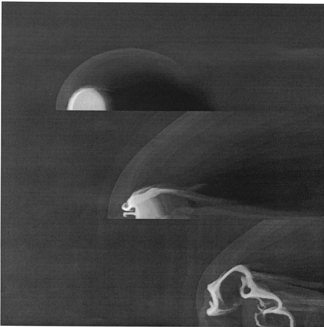
FIG. 1.—Numerical simulation of density distribution in a supersonic clump at three time steps characterizing the major phases of dynamical evolution: ( top ) the bow-shock phase, ( middle ) the instability phase, and ( bottom ) the dispersal phase. The clump began with a density contrast \chi = 100 and also was stationary in the grid, with the ambient medium flowing at Mach 10 from left to right. Times shown correspond to t/t_{bc} \approx 0.2, 1.5, and 2.5 . The gray scale is logarithmic, with lightest tones about 400 times the ambient density. Eighty-five numerical zones were contained by one original clump diameter. The computation was two-dimensional on a Cartesian grid. Other computational details can be found in JKT (their model 2) and Jones & Kang (1993).
