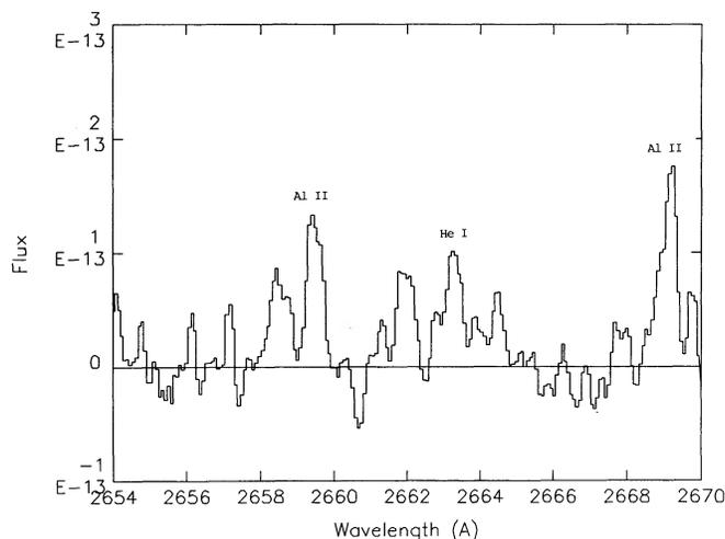
FIG. 2.—High-resolution 300 minute *IUE* spectrum (LWR 2571) of the planetary nebula NGC 7027 in the wavelength region 2654–2670 Å, where the flux is in units of  $\text{ergs cm}^{-2} \text{ s}^{-1}$ . The Al II  $3s^2^1S-3s3p^3P_2$  and  $3s^2^1S-3s3p^3P_1$  transitions at 2660 and 2669 Å, respectively, are clearly labeled in the figure.
