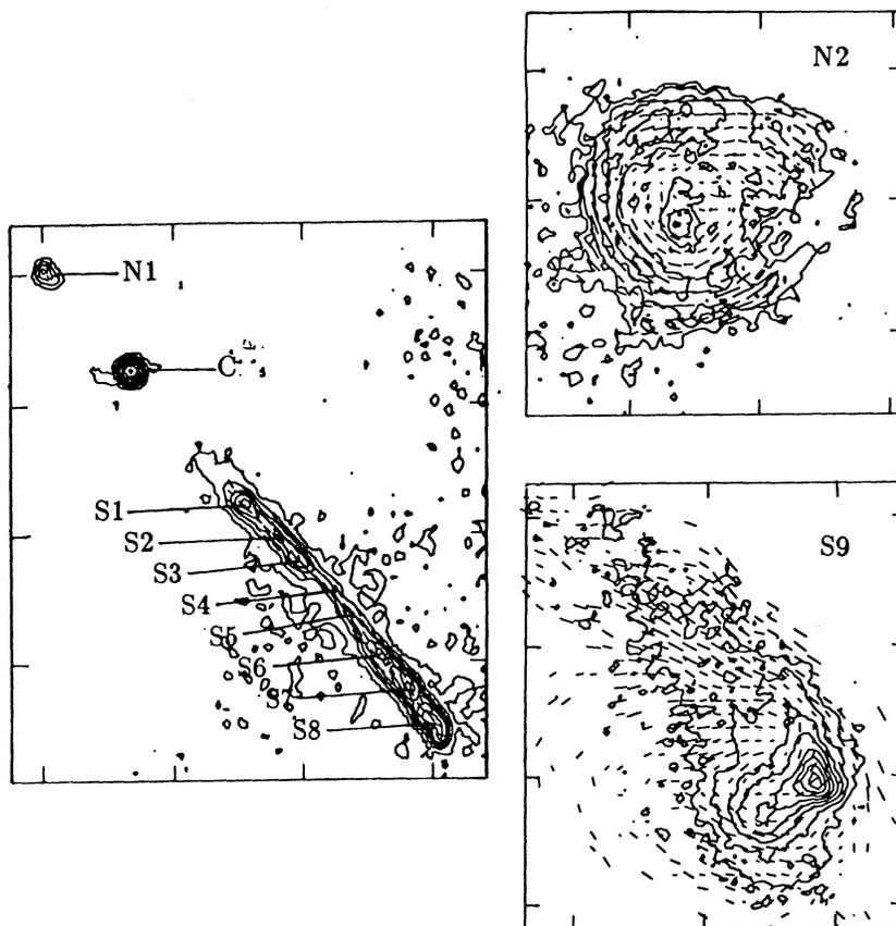
FIG. 9.—Montage of 6 cm, 0.4 resolution images of fractional polarization  $B$ -vectors superposed over total intensity contours of the northern hot spot (top right), the jet-core region (left), and the southern hot spot (bottom right). The angular distance between the tick marks around the perimeter of each image is 5".
