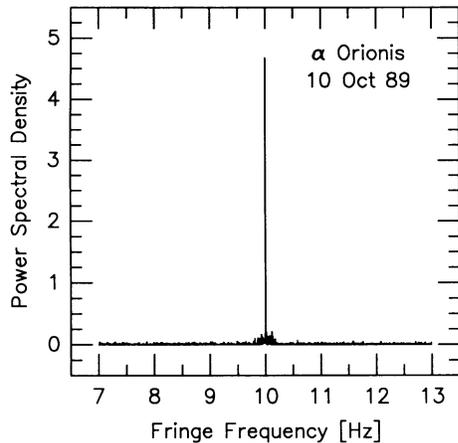
FIG. 1.—Power spectrum of interference fringes of  $\alpha$  Orionis, taken on 1989 October 10. This fringe spectrum represents 5.5 minutes of observation and is kept at 10 Hz by lobe rotation. The central spike has a frequency width equal to the inverse of the observing time, or 3.0 mHz; sidebands are due to atmospheric fluctuations.
