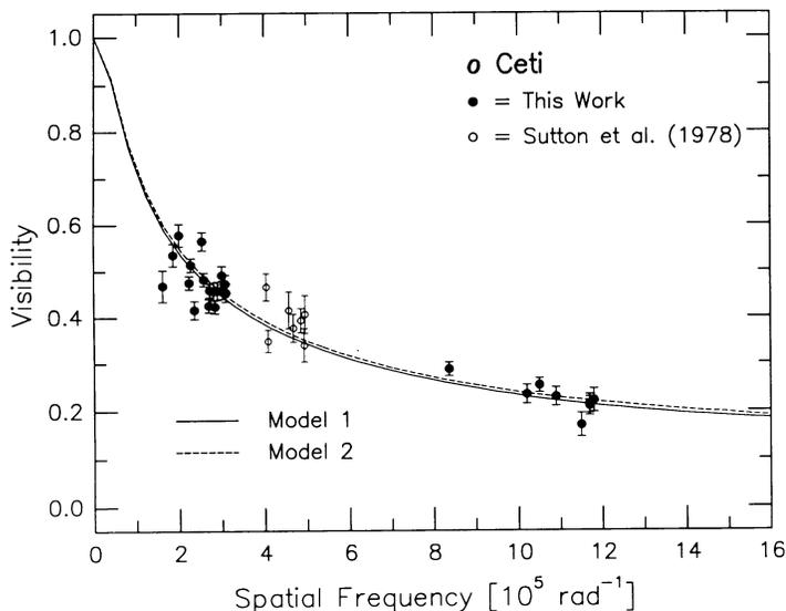
FIG. 2.—Visibilities of  $\alpha$  Ceti as a function of spatial frequency near maximum of the LPV's luminosity cycle. The data include our measurements made between 1989 October 10 and December 5 and, in the spatial frequency range  $4\text{--}5 \times 10^5 \text{ rad}^{-1}$ , data of Sutton et al. (1978) taken near maximum luminosity in 1978 January. The solid curve represents predictions from model 1 of Table 1 and the dashed curve those from model 2; both are acceptable fits to the data.
