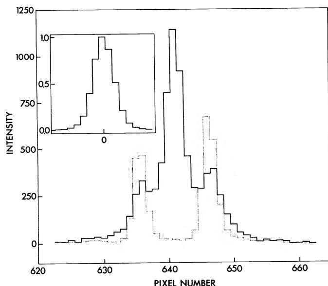
FIG. 2.—The flux (in arbitrary units) from the raw  $\lambda 5008$  image of SN 1987A as a function of position along an E-W line centered on the SN (solid line). The dotted line shows a similar cut through the image after processing to remove the stellar images and deconvolving the nebular image with a point-spread function obtained from field stars in the same frame. The point-spread function is shown in the upper left box. One pixel corresponds to  $0''.152$ . East is to the left.
