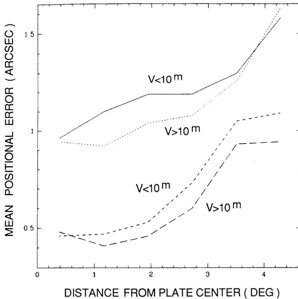
FIG. 4.—As in Fig. 1 but each hemisphere has been split into two mutually exclusive magnitude groups at  $V = 10 \text{ mag}$ . For each of the two pairs of curves, the fainter sample is the lower one.
