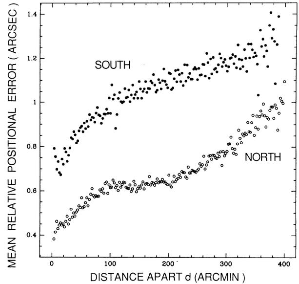
FIG. 5.—(Total) positional error for a single star based on the relative errors for pairs of stars (on the same plate) as a function of separation. Points for the south are filled circles; points for the north are open circles.
