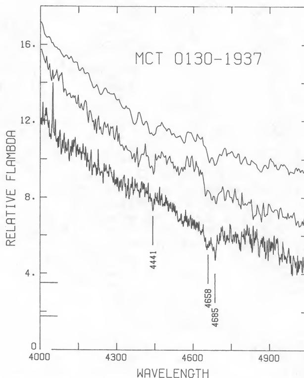
FIG. 2.—Optical spectra of MCT 0130–1937. These are, from top to bottom, our discovery SIT scan at  $13.5 \text{ \AA}$  resolution; a CTIO 1.5 m spectrum at  $8 \text{ \AA}$  resolution; and a Steward Observatory 2.3 m spectrum at  $2.5 \text{ \AA}$  resolution. The C iv feature at 4441  $\text{\AA}$  and the characteristic C iv  $\lambda 4658$ –He II  $\lambda 4686$  blend are indicated.
