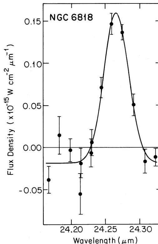
FIG. 1.—Grating spectrometer spectrum of NGC 6818 taken aboard the Kuiper Airborne Observatory on 1984 May 22. A Gaussian instrumental function is fitted to the [Ne v]  $24.3 \mu\text{m}$  line. The wavelength resolution (FWHM) was determined from other data and is  $0.04 \mu\text{m}$ .
