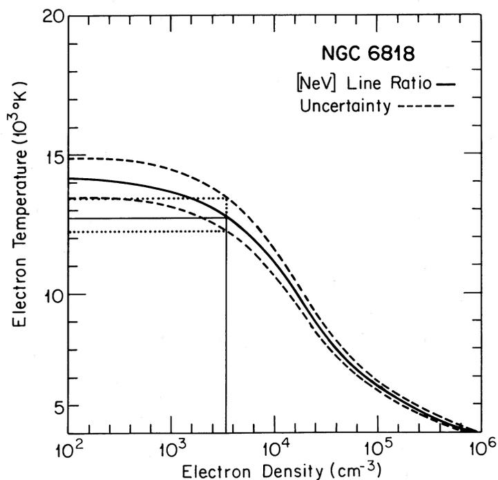
FIG. 4.—A plot of the  $[\text{Ne V}] I(24.3 \mu\text{m})/I(3426 \text{ \AA})$  ratio for NGC 6818 (*Solid line*). The uncertainty ( $1 \sigma$ ) in the ratio is indicated by the broken lines. This ratio constrains the range of  $T_e$  and  $n_e$  values in the Ne v zone. Taking a density of  $3500 \text{ cm}^{-3}$  (as indicated on the plot) that has been derived from optical forbidden lines (see text) a Ne v electron temperature of  $12.700^{+800}_{-300} \text{ K}$  is found.
