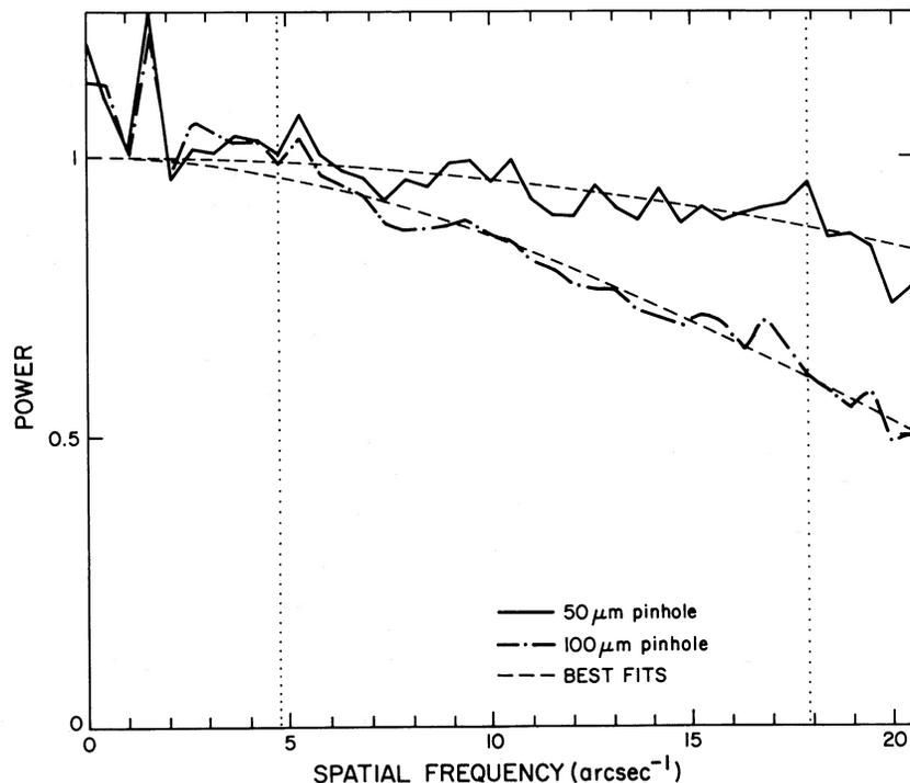
FIG. 2.—Laboratory simulation power spectra and best-fit Airy disks for the 50 and 100  $\mu\text{m}$  pinholes. Vertical dotted lines show the range of fitted region. The diffraction limit of the optical system at 6563  $\text{\AA}$  was  $30 \text{ arcsec}^{-1}$ .
