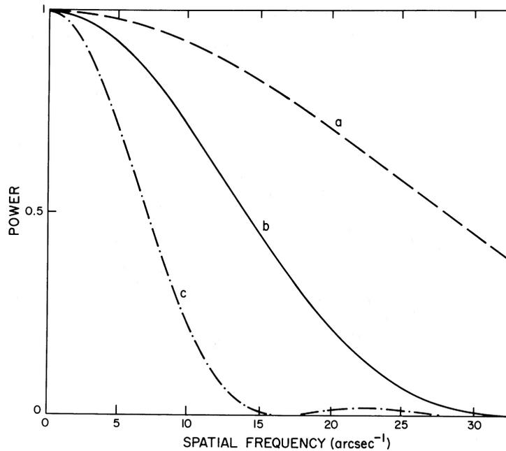
FIG. 1.—Ideal power spectra for stars with diameters (a) 0.5, (b) 1, and (c) 2 times the telescope diffraction limit. The right-hand axis corresponds to the 4 m diffraction limit at 6000 Å (33 arcsec<sup>-1</sup>).
