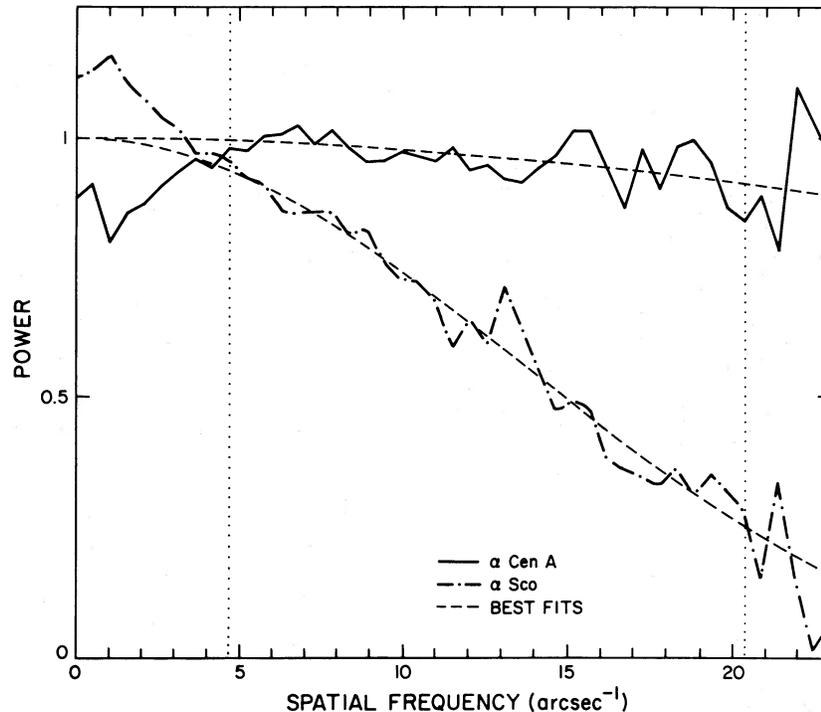
FIG. 3.—Power spectra for  $\alpha$  Cen A and  $\alpha$  Sco, stars with known diameters. The best fits to the data (corresponding to a uniform disk of 9 mas for  $\alpha$  Cen A and 35 mas for  $\alpha$  Sco) are also plotted. Vertical dotted lines show the range of fitted region.
